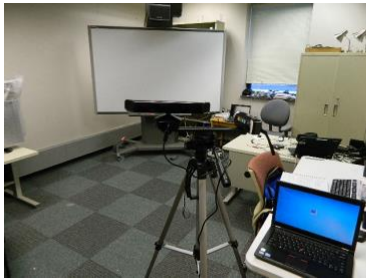
Figure 1: Apparatus and setting of the data collection. A Microsoft V1 Kinect and a JVC camcorder were mounted together on a tripod. The laptop in the foreground runs the Brekel program for recording motions. The smartboard and the other laptop (away from the readers) were used to present slides for the B and C tasks.
